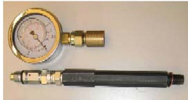
Cylinder compression gauge item no 4786-167-000
