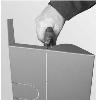
Fig.26 Cut through lever at top and bottom
