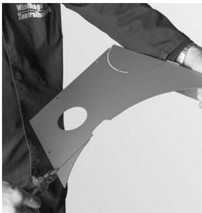
Fig.30 Pinch off the corner of the cladding at top left
