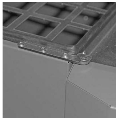
Fig.39 Screw the door hinge and fitted cladding door into position
