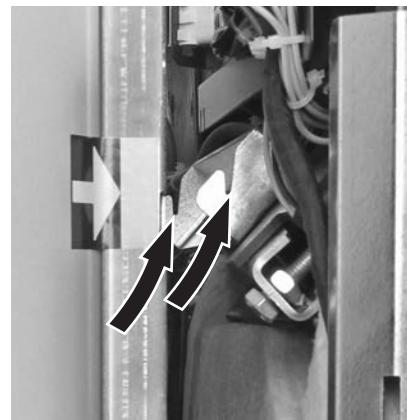
Fig.11 Suspend hopper from 2 hooks, as marked
