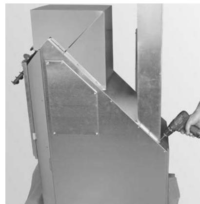
Fig. 7 Remove 6 screws
