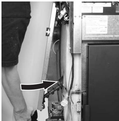
Fig. 9 Insert auger conveyor into bottom of auger tube
