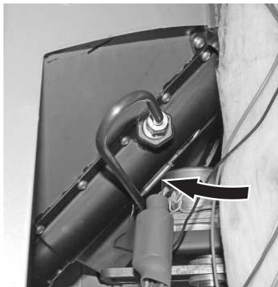
Fig. 14 Insert sensor for safety thermostat auger tube as far as possible
