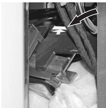
Fig. 11 Tighten fastening at top as firmly as possible (as marked)
