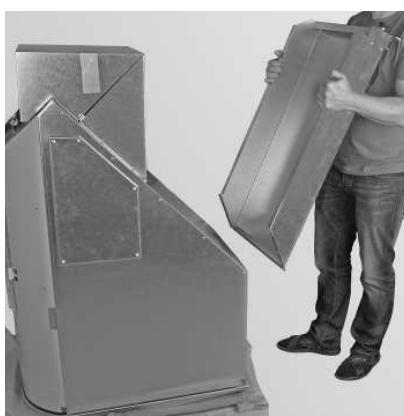
Fig. 7 Remove pedestal
