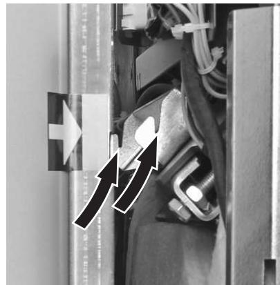
Fig. 10 Suspend hopper from 2 hooks, as marked
