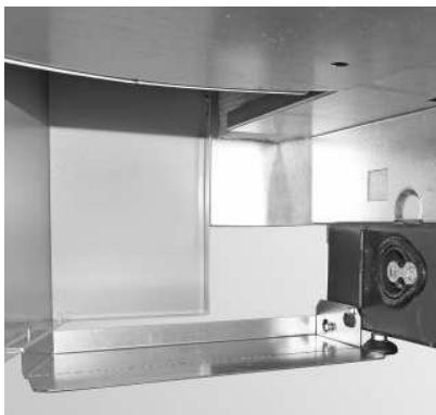
Fig. 39 Fit the ash box base
