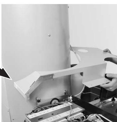
Fig. 31 Position cladding carefully at top left
